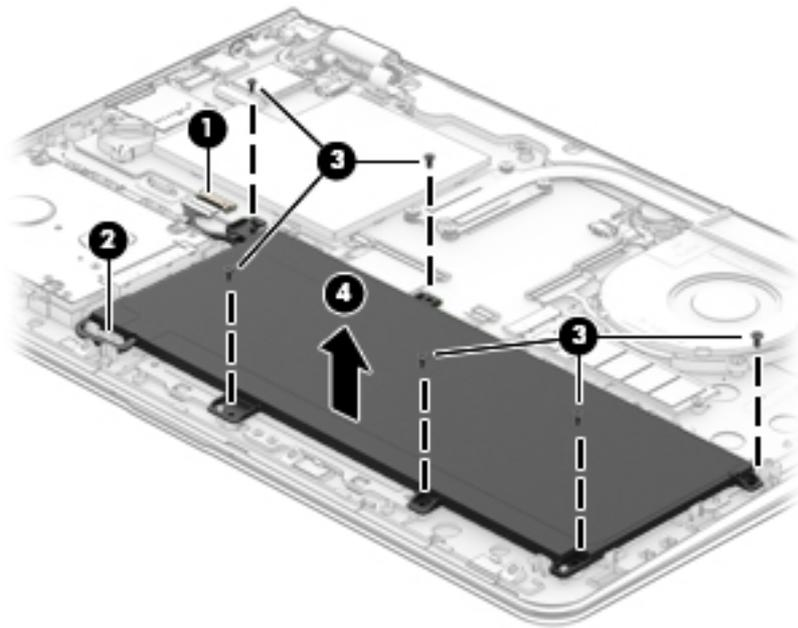
Reverse this procedure to install the battery.
