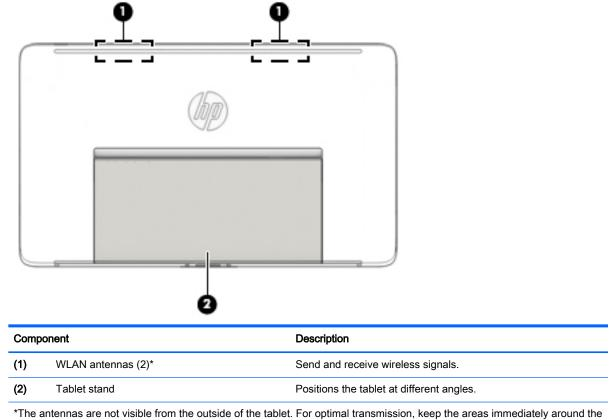
\*The antennas are not visible from the outside of the tablet. For optimal transmission, keep the areas immediately around the antennas free from obstructions. For wireless regulatory notices, see the section of the *Regulatory, Safety, and Environmental Notices* that applies to your country or region. To access this guide, from the Start screen, type support, and then select the **HP Support Assistant** app.
