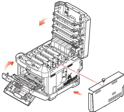
9. Close the front cover and the top cover, pressing down firmly at each side to latch it closed.
