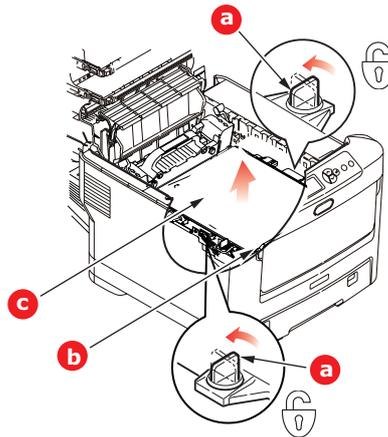
5. Turn the two fasteners 90° to the left. This will release the belt from the printer chassis.
