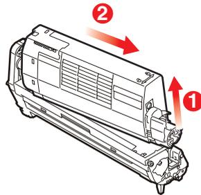
7. Take the new image drum cartridge out of its packaging and place it on the piece of paper where the old cartridge was placed. Keep it the same way round as the old unit. Pack the old cartridge inside the packaging material for disposal.
