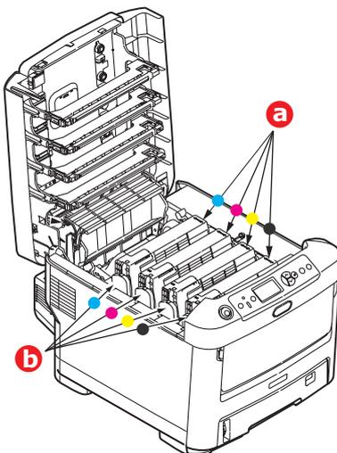
3. Lift each of the image drum units out of the printer and place them in a safe place away from direct sources of heat and light.
