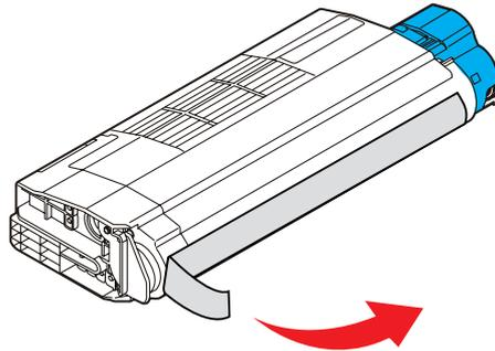
8. Holding the cartridge by its top centre with the coloured lever to the right, lower it into the printer over the image drum unit from which the old cartridge was removed.
