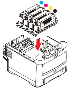
Holding the complete assembly by its top centre, lower it into place in the printer, locating the pegs at each end into their slots in the sides of the printer cavity.
