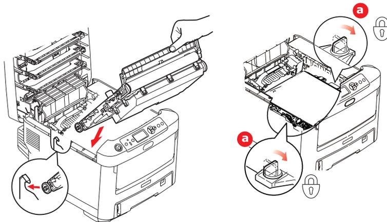
8. Turn the two fasteners (a) 90° to the right until they lock. This will secure the belt unit in place.
