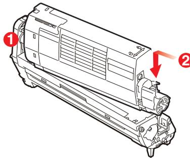
9. Push the coloured release lever away from you to lock the toner cartridge onto the new image drum unit and release toner into it.
