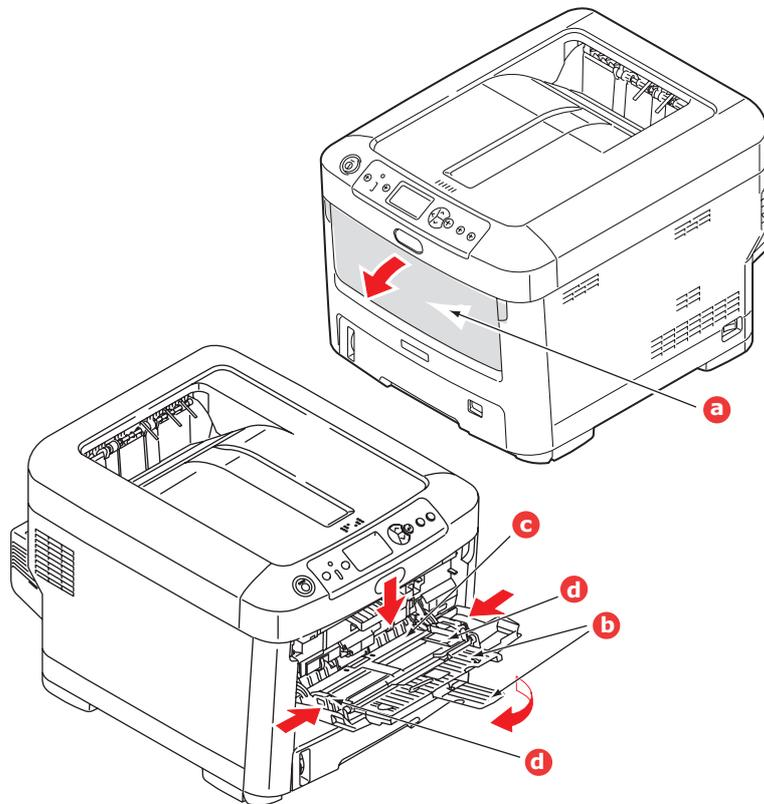
3. Press gently down on the paper platform (c) to ensure it is latched down.
