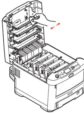
12. Finally, close the top cover and press down firmly at both sides so that the cover latches closed.
