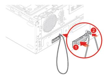
Figure 78. Installing the front Wi-Fi antenna
