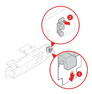
Figure 104. Installing the power button
