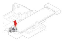
Figure 57. Unlocking the M.2 solid-state drive clip
