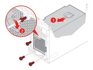
Figure 75. Installing the power supply assembly
