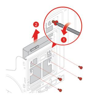
Figure 31. Removing the 3.5-inch primary storage drive
