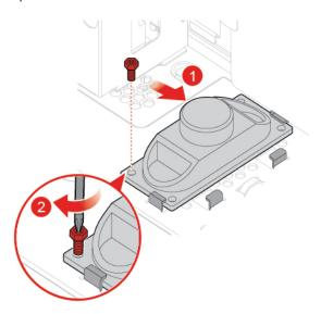
Figure 85. Installing the internal speaker
