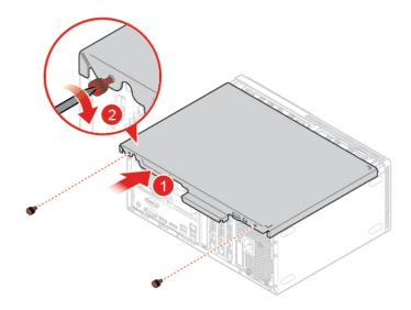
Figure 135. Reinstalling the computer cover
