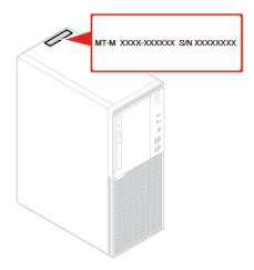
Figure 4. Machine type and model label
