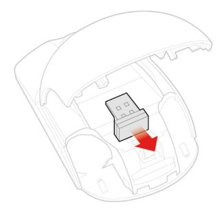
Figure 14. Taking out the USB dongle
