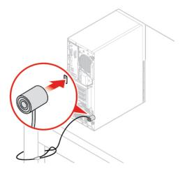
Figure 7. Attaching a Kensington-style cable lock
