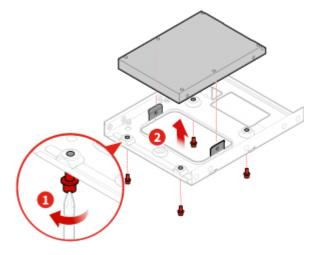
Figure 38. Removing the 2.5-inch storage drive from the storage converter
