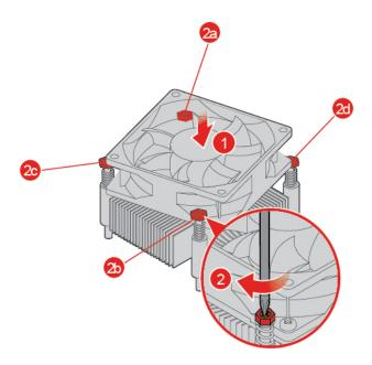
Figure 109. Installing the heat sink and fan assembly
