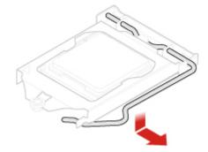
Figure 112. Unlocking the microprocessor socket retainer
