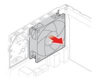
Figure 131. Removing the rear fan
