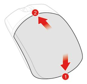
Figure 17. Closing the battery compartment cover
