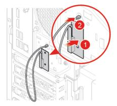
Figure 81. Installing the rear Wi-Fi antenna
