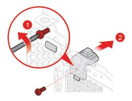
Figure 127. Removing the cover presence switch
