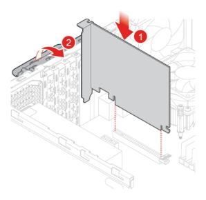
Figure 47. Installing the PCI Express card
