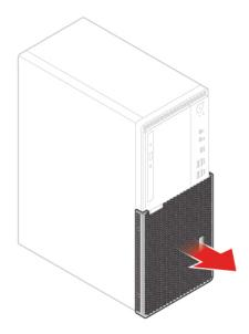
Figure 21. Removing the dust shield
