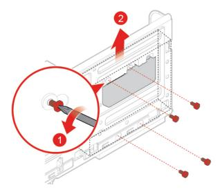
Figure 35. Removing the 3.5-inch secondary storage drive
