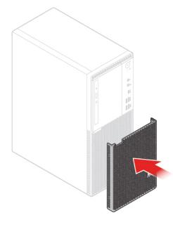
Figure 22. Installing the dust shield
