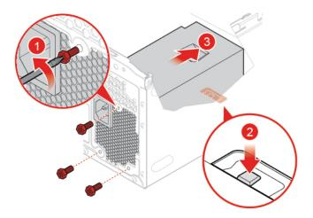
Figure 74. Removing the power supply assembly
