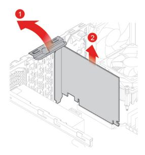
Figure 46. Removing the PCI Express card
