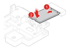
Figure 67. Installing the M.2 solid-state drive
