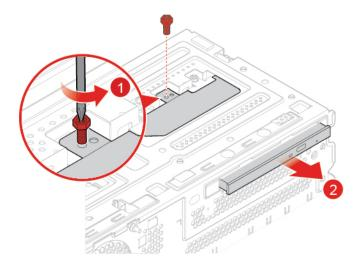
Figure 26. Removing the optical drive
