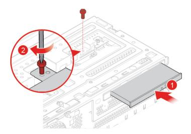
Figure 27. Installing the optical drive
