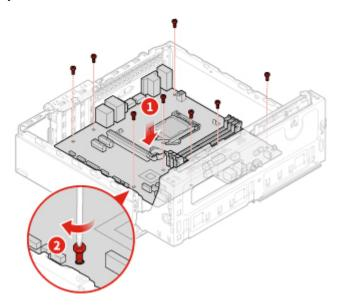
Figure 134. Installing the system board
