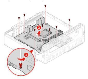
Figure 133. Removing the system board
