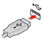
Figure 12. Replacing the mouse
