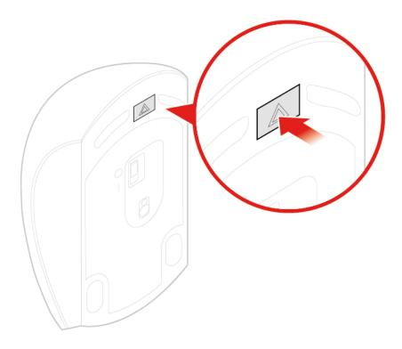
Figure 13. Opening the battery compartment
