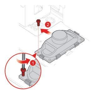
Figure 84. Removing the internal speaker
