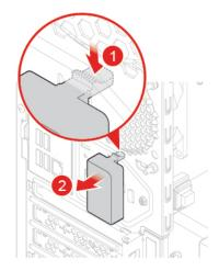
Figure 79. Removing the rear Wi-Fi antenna cover
