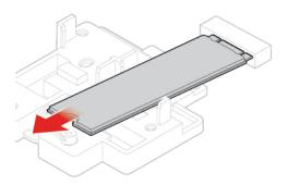
Figure 58. Removing the M.2 solid-state drive
