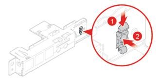
Figure 103. Removing the power button
