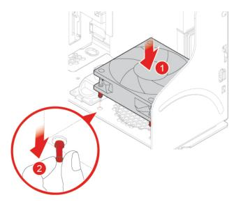
Figure 89. Installing the front fan
