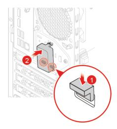
Figure 82. Installing the rear Wi-Fi antenna cover
