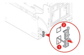
Figure 97. Installing the thermal sensor
