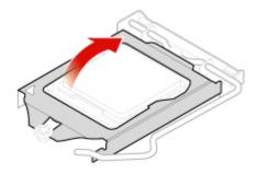
Figure 113. Pivoting the microprocessor socket upward
