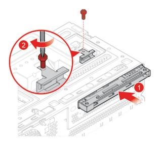
Figure 29. Installing the optical drive bracket
