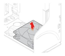
Figure 88. Removing the front fan
