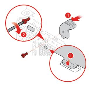
Figure 128. Installing the cover presence switch
