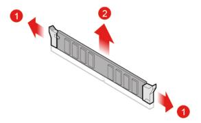
Figure 42. Removing the memory module
