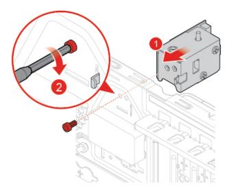
Figure 126. Installing the E-lock
