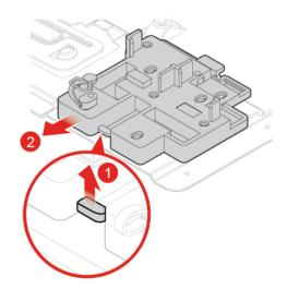
Figure 71. Removing the M.2 solid-state drive bracket
