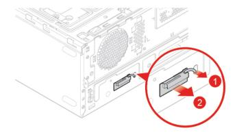
Figure 77. Removing the front Wi-Fi antenna
