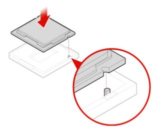
Figure 115. Installing the microprocessor
