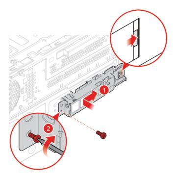
Figure 101. Installing the front I/O bracket
