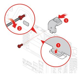
Figure 130. Installing the cover presence switch
