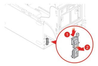
Figure 96. Removing the thermal sensor
