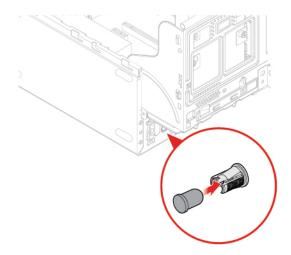
Figure 93. Installing the illuminated red dot cable
