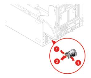
Figure 92. Removing the illuminated red dot cable
