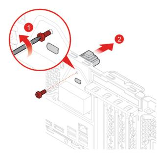
Figure 129. Removing the cover presence switch
