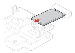
Figure 66. Removing the M.2 solid-state drive
