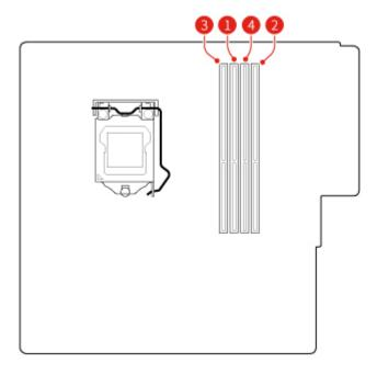
Figure 40. Installation order for memory modules
