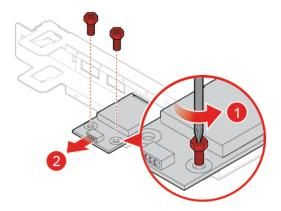
Figure 105. Removing the card reader board
