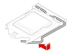
Figure 117. Locking the microprocessor socket retainer
