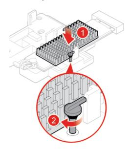
Figure 61. Installing the M.2 solid-state drive heat sink
