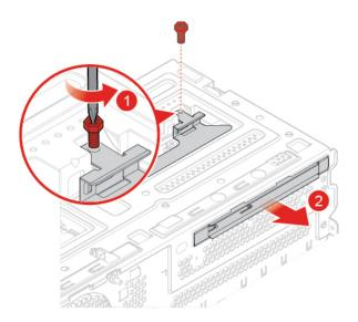
Figure 28. Removing the optical drive bracket
