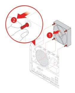
Figure 132. Installing the rear fan
