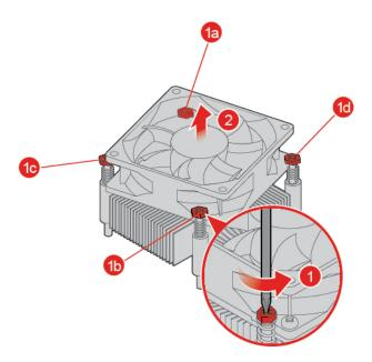
Figure 108. Removing the heat sink and fan assembly
