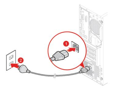
Figure 20. Installing the power cord
