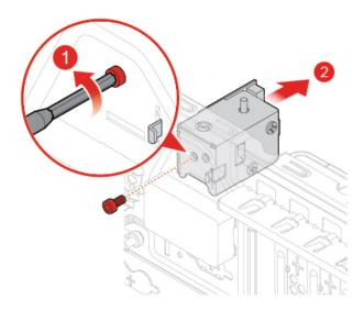
Figure 125. Removing the E-lock
