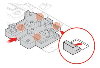
Figure 72. Installing the M.2 solid-state drive bracket
