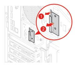
Figure 80. Removing the rear Wi-Fi antenna
