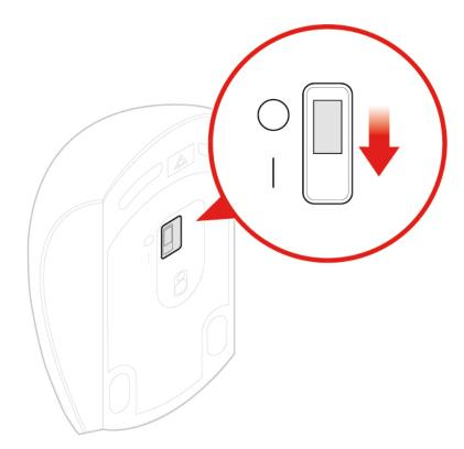
Figure 18. Pushing the power switch to the on position
