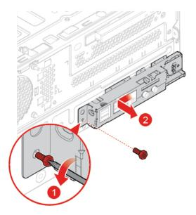
Figure 100. Removing the front I/O bracket
