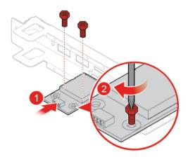
Figure 106. Installing the card reader board
