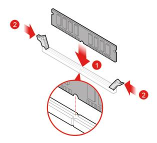
Figure 43. Installing the memory module
