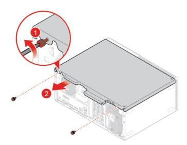
Figure 23. Removing the computer cover
