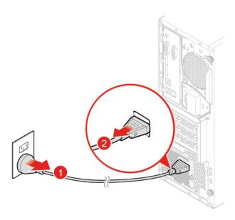
Figure 19. Removing the power cord
