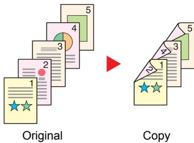
Produces two-sided copies from one-sided originals. In case of an odd number of originals, the back side of the last copy will be blank.
