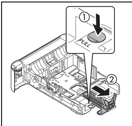
If you are going to use paper that is longer than A4-R, pull the cassette out until it stops at the back and then adjust the paper length guide to the paper size required.
