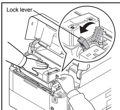
**2** Turn the lock lever to the unlock position.
