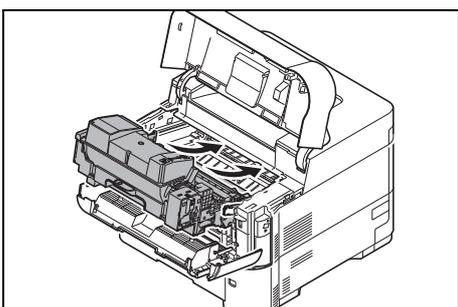
**4** Insert the developer unit together with the toner container, back into the machine.
