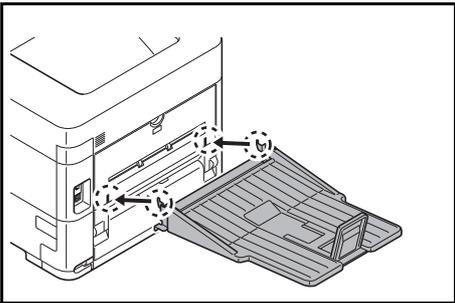
**2** Install the faceup output tray on the rear of the printer.
