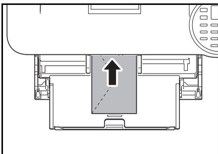
Envelopes should be fed from the MP tray with the print-side up or the optional paper feeder (PF-320) with the print-side down.
