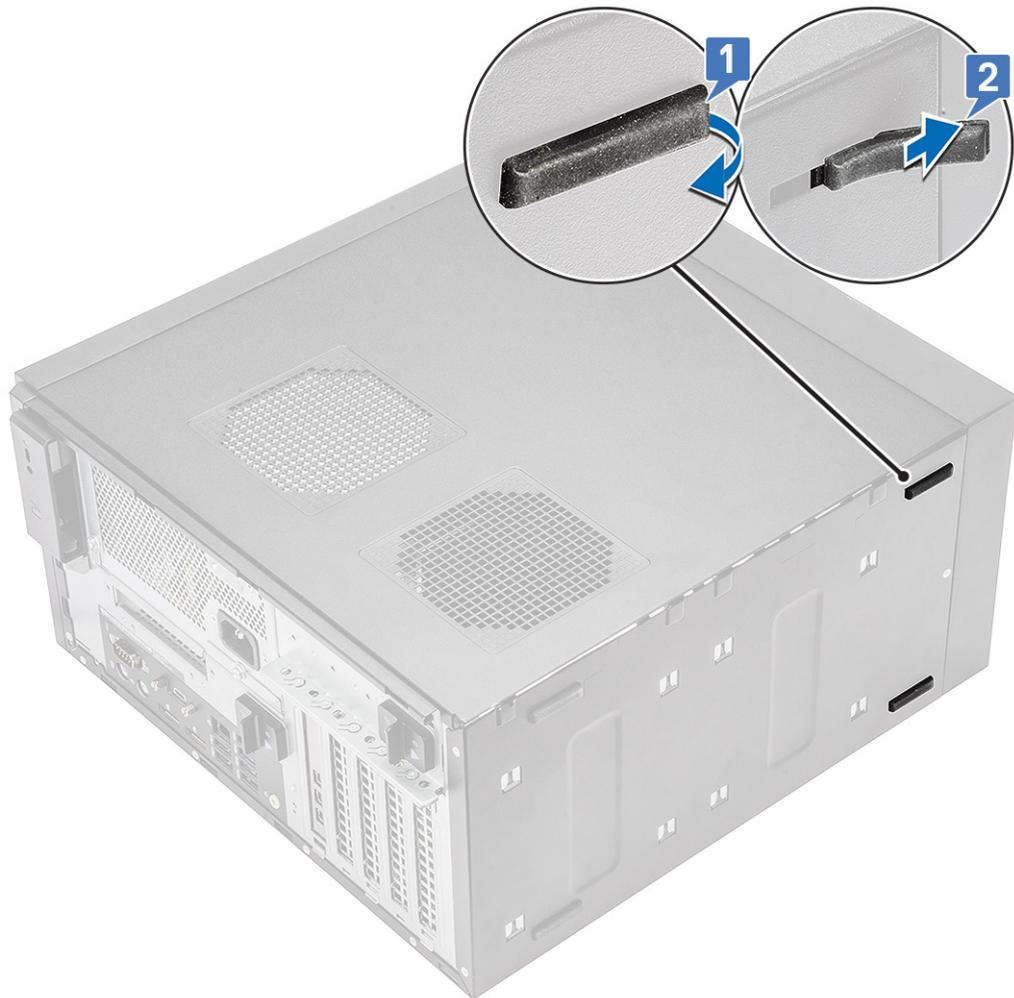
Figure 4. Front rubber feet removal
