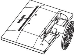
2. Press the locking clips to detach the base stand away from the base column.
