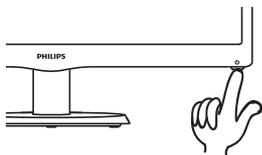
2. Turn on the monitor by pressing the bottom key once.
