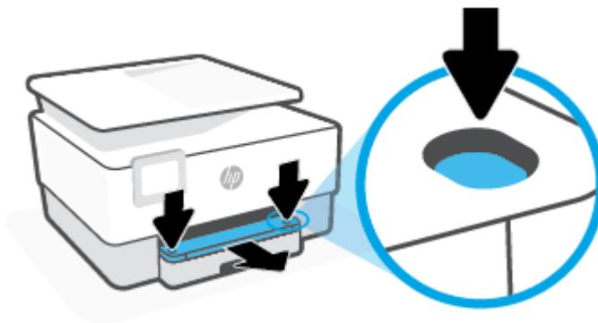
2. Remove the input tray by pulling it all the way out of the printer.
