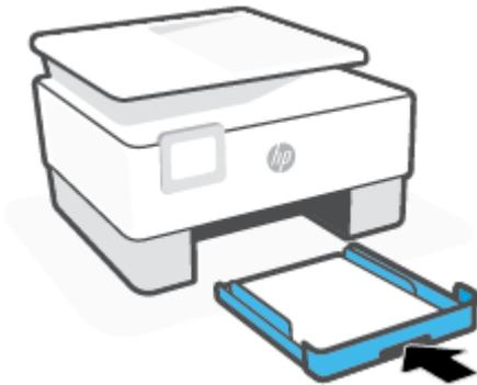
5. Insert the output tray back into the printer.
