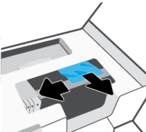
4. If need, move the carriage to the far right of the printer, and remove any jammed or torn pieces of paper.
