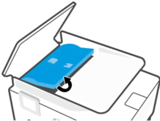
4. Pull any jammed paper out under the rollers.
