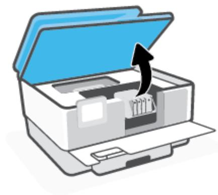
3. If the print carriage is not obstructed, move the print carriage to the far left of the printer and remove the jammed paper.
