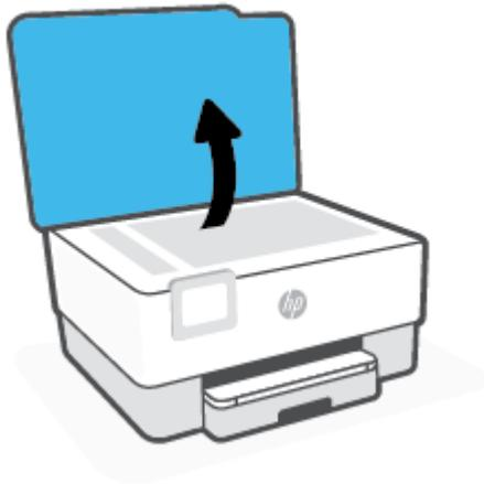
2. Clean the scanner glass and lid backing by using a soft, lint-free cloth that has been sprayed with a mild glass cleaner.
