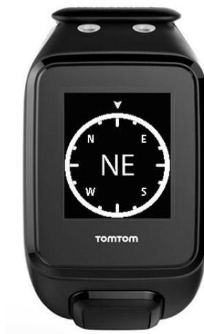
The compass works best when the watch is kept level. If the compass doesn't show the correct direction, you need to [calibrate the compass](#).
