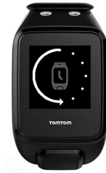
Repeat steps a-c until the compass is calibrated. When calibrated the watch gives an alert and shows a tick.
