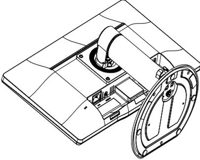
2. Use a flathead screwdriver to remove four mylars from the hinge cover.
