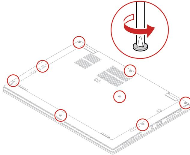
6. Pry up the latches and remove the base cover assembly.
