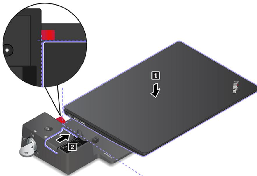
5. Check the docking status indicator. The docking status indicator turns on when the computer is successfully docked.
