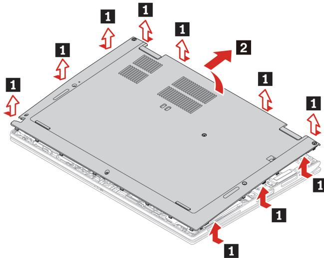
7. Install the new base cover assembly in place. Ensure that the latches of the base cover assembly are secured under the base cover assembly.
