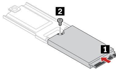
8. Align the contact edge of the new M.2 solid-state drive with the key in the slot. Then, carefully insert the drive with the bracket into the slot **1**. Tighten the screw **2**.
