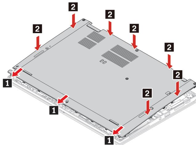
8. Tighten the screws to secure the base cover assembly.
