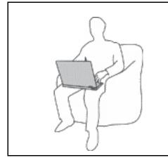
When your computer is turned on or the battery is charging, the base, the palm rest, and some other parts may become hot. The temperature they reach depends on the amount of system activity and the level of charge in the battery.
