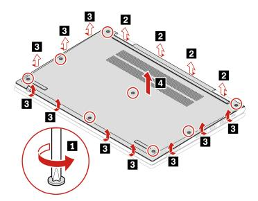
5. Install the new base cover assembly in place. Ensure that the latches of the base cover assembly are secured under the base cover assembly. Then, tighten the screws to secure the base cover assembly.
