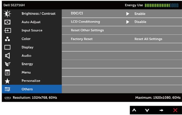
Select this option to adjust the OSD settings, such as the **DDC/CI**, **LCD conditioning**, and so on.
