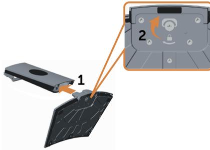
Attach the stand assembly to the monitor.
