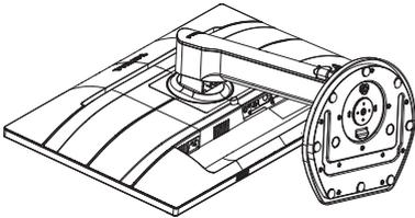
3. While keeping the release button pressed, tilt the base and slide it out.
