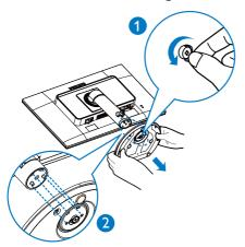
3. While keeping the release button pressed, tilt the base and slide it out.
