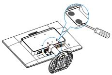
3. Remove the screws from hinge cover.
