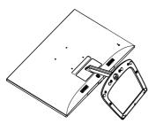
2. Use your fingers to loosen the screw located at the bottom of the base, and remove the base from the stand.
