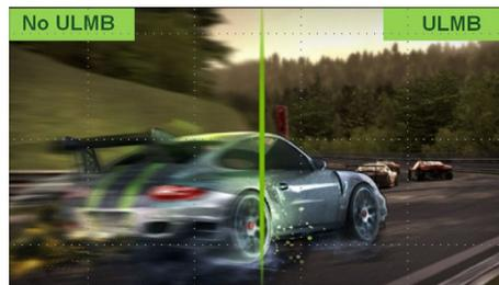
With NVIDIA Ultra Low Motion Blur (ULMB) mode, objects in motion look sharper than they do during standard operation-even at high refresh rates such as 120Hz.
