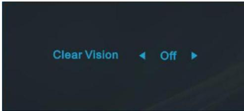
3. Press and hold “<” button for 5 seconds to activate the Clear Vision Demo, and a message of “Clear Vision Demo: on” will be display on the screen for a duration of 5 seconds. Press Menu or Exit button, the message will disappear. Press and hold “<” button for 5 seconds again, Clear Vision Demo will be off.
