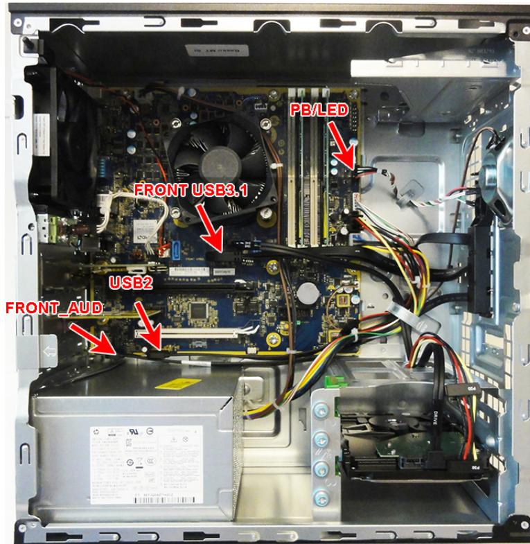
7. Remove the front I/O and power switch assembly from the inside of the computer.
