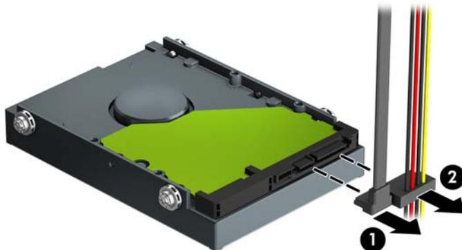
4. Pull the green latch next to the drive outward **(1)** and slide the drive out of the bay **(2)**.
