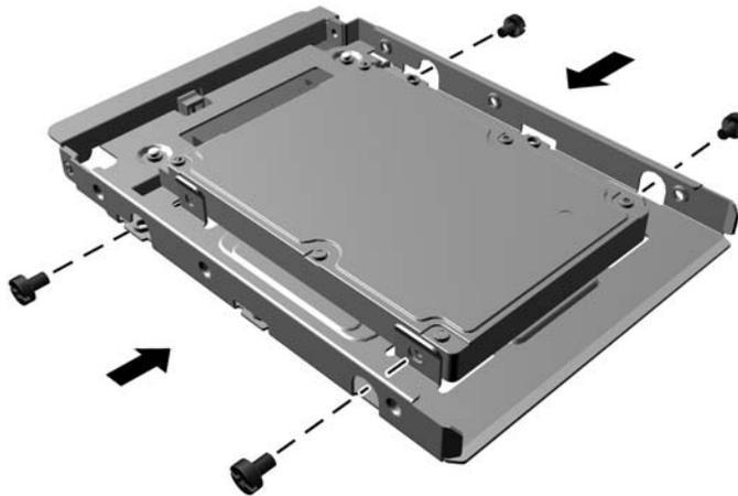
4. Install four mounting screws into the sides of the 3.5-inch drive or the 2.5-inch drive adapter bracket (two on each side).
