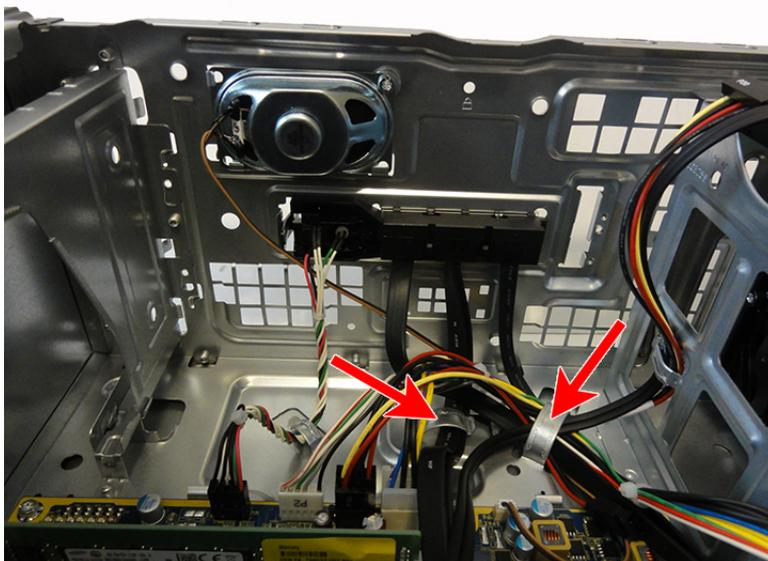
6. Disconnect the four cables from the following system board connectors:
