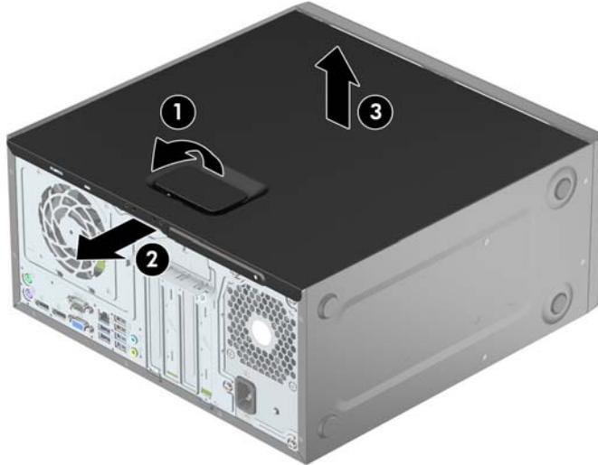
To replace the access panel, reverse the disassembly procedures.
