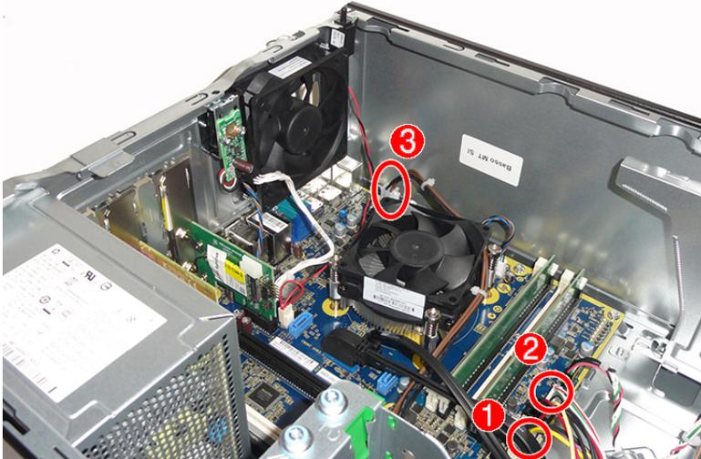
6. Press the tab (1) on the base pan in front of the power supply that holds it in place.
