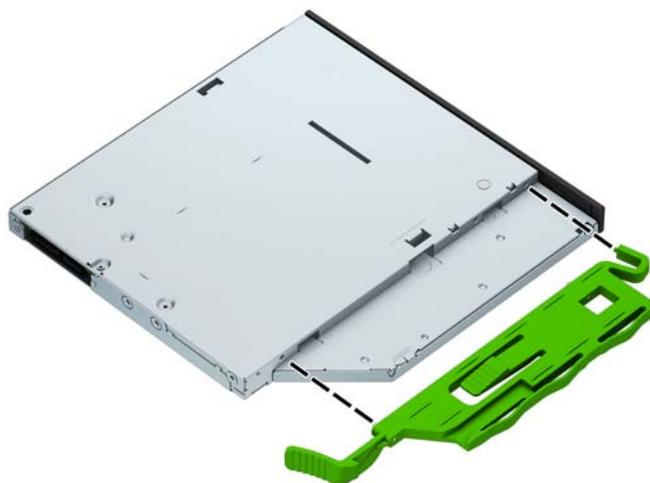
6. Slide the optical drive through the front of the chassis (1) all the way into the bay so that the green latch locks onto the chassis frame (2).
