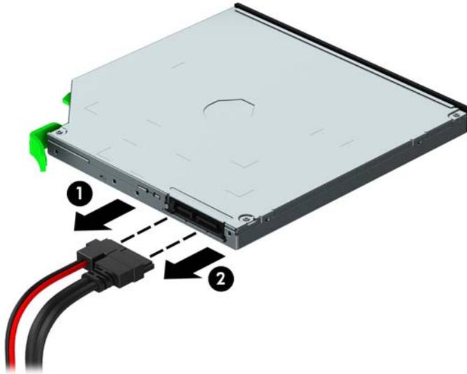
**CAUTION:** When removing the cables, pull the tab or connector instead of the cable itself to avoid damaging the cable.
