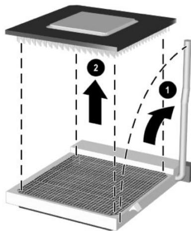
Reverse the removal procedure to install a new processor.
