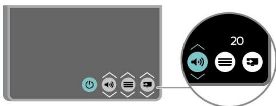
Press up or down to adjust the volume or tune to the next or previous channel. Press up or down to go through the list of sources, including the tuner selection.
