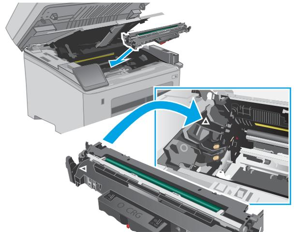
9. Align the toner cartridge with the tracks inside the printer, and install the toner cartridge until it is firmly seated.
