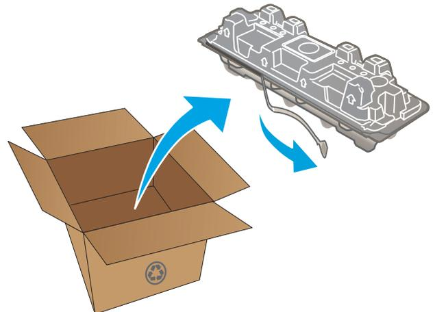
5. Remove the new toner cartridge from the opened packaging shell. Place the used toner cartridge in the shell for recycling.
