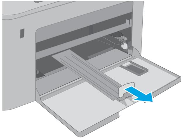
4. Load the paper into the tray. For information about how to orient the paper, see [Main input tray paper orientation on page 24](#).
