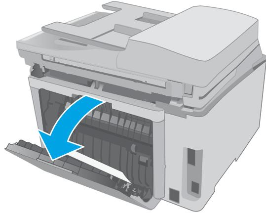
2. Remove any jammed paper from the duplex area. Use both hands to remove jammed paper to avoid tearing the paper.
