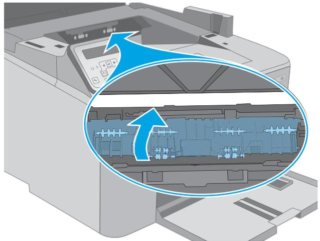
10. Align the imaging drum with the tracks inside the printer, and install the imaging drum until it is firmly seated.
