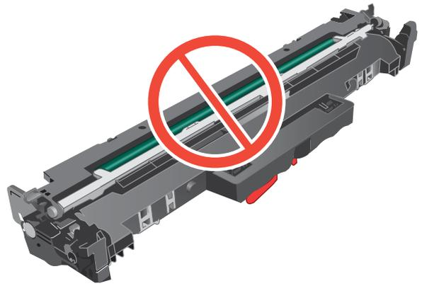
8. Align the new imaging drum with the tracks inside the printer, and install the new imaging drum until it is firmly seated.
