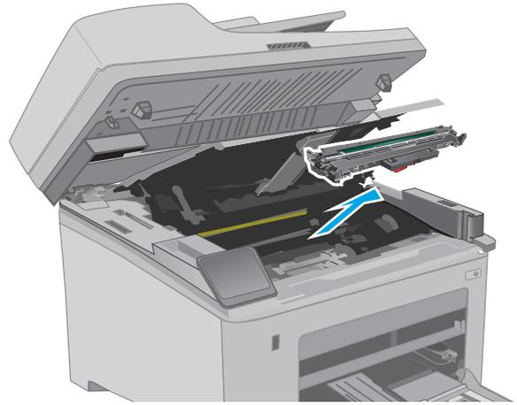
5. Remove the new imaging drum package from the box, and then release the packaging.
