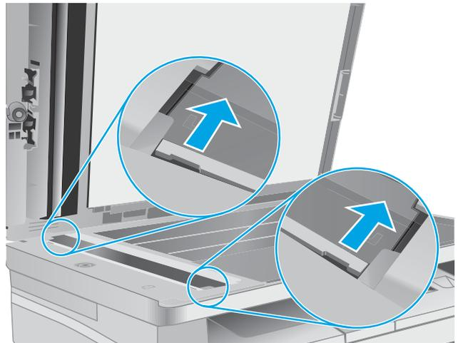
3. Slide the assembly in the direction indicated to remove it.
