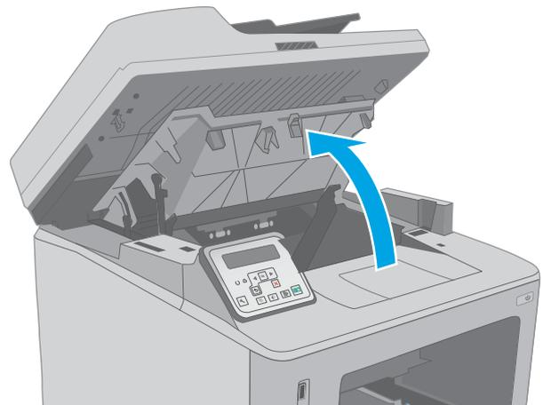
4. Remove the toner cartridge from the printer.
