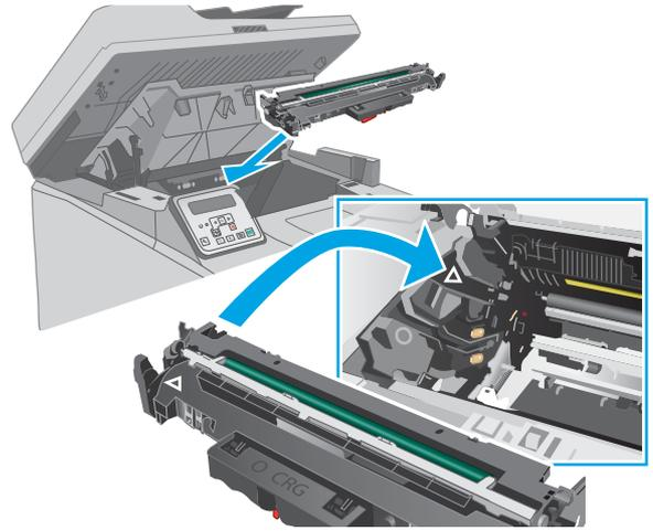
11. Align the toner cartridge with the tracks inside the printer, and install the toner cartridge until it is firmly seated.
