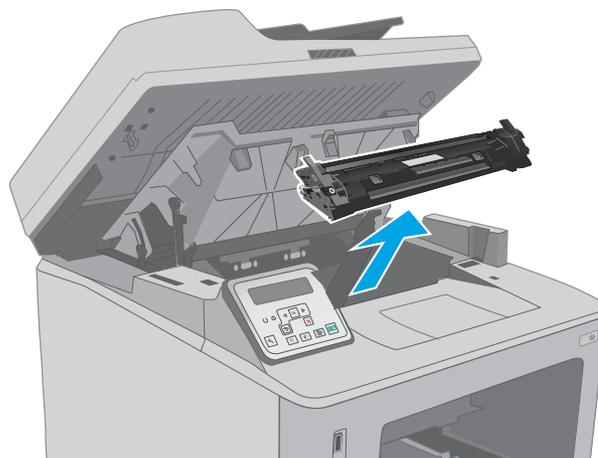
4. Remove the imaging drum from the printer.
