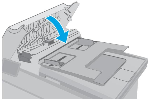
6. Open the scanner lid. If paper is jammed behind the white plastic backing, gently pull it out.
