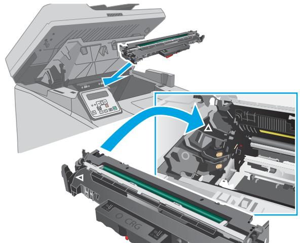
10. Align the toner cartridge with the tracks inside the printer, and install the toner cartridge until it is firmly seated.
