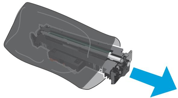
7. Do not touch the imaging drum. Fingerprints on the imaging drum can cause print-quality problems.
