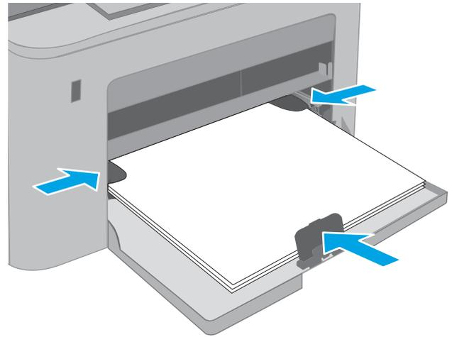
6. If the paper is A4 size, Letter-size or smaller, close the Main input tray door. Use the paper-stack window to verify that is correctly loaded.
