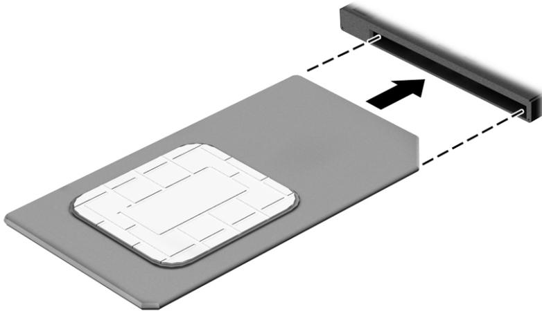
To remove a SIM card, press in on the SIM card, and then remove it from the slot.
