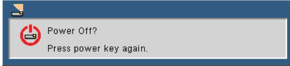
2. Press the "POWER" button again to confirm. When the light turns red, the projector has entered standby mode.
