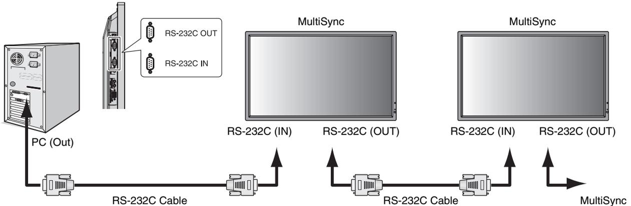
**NOTE:** If your PC is equipped only with a 25-pin serial port connector, a 25-pin serial port adapter is required. Contact your dealer for details.
