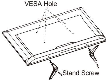
1. Loosen the screws on the button of the base, and remove the base.
