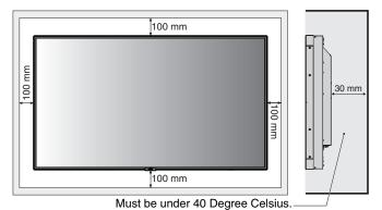
Allow adequate ventilation or provide air conditioning around the monitor, so that heat can properly dissipate away from the unit and mounting equipment; especially when you use monitors in multiple screen.
