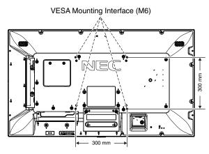
Mounting accessories can be attached with the monitor in the face down position. To avoid damaging the screen face, place the protective sheet on the table underneath the LCD. The protective sheet was wrapped around the LCD in the original packaging. Make sure there is nothing on the table that can damage the monitor.
