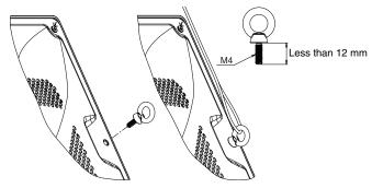
Using wire with LCD monitor optional speaker installed.
