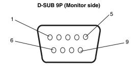
This LCD monitor uses RXD, TXD and GND lines for RS-232C control.
