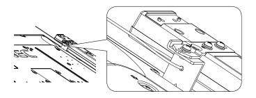
Optional speaker is installed on the side of the LCD monitor:
