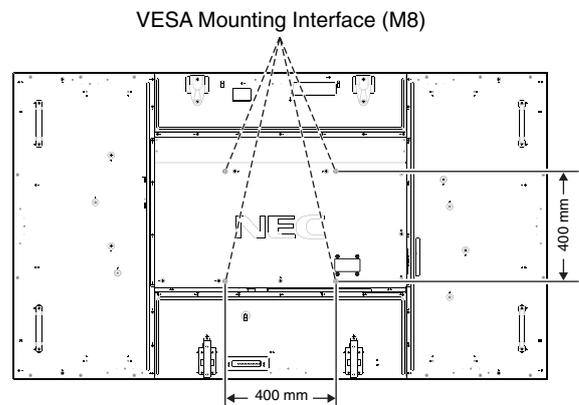
Mounting accessories can be attached with the monitor in the face down position. To avoid damaging the screen face, place the protective sheet on the table underneath the LCD. The protective sheet was wrapped around the LCD in the original packaging. Make sure there is nothing on the table that can damage the monitor.
