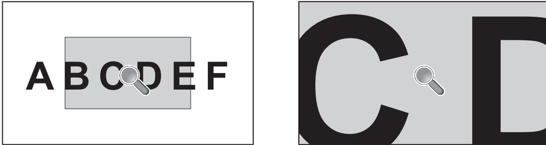
Using “SET/POINT ZOOM” button on a remote control allows to enlarge a partial of image. Press CH+/- button to zoom up or down. The image can be expanded from 1 to 10 times.
