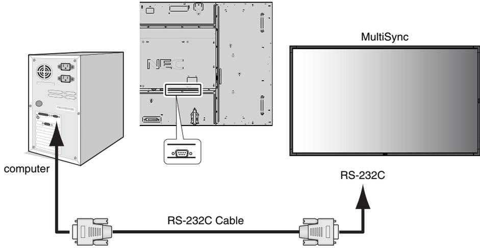
**NOTE:** If your computer is equipped only with a 25-pin serial port connector, a 25-pin serial port adapter is required. Contact your dealer for details.
