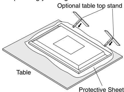
**NOTE:** Install the stand in the direction of the arrow which is imprinted on the surface of the stand. Use the ST-801.
