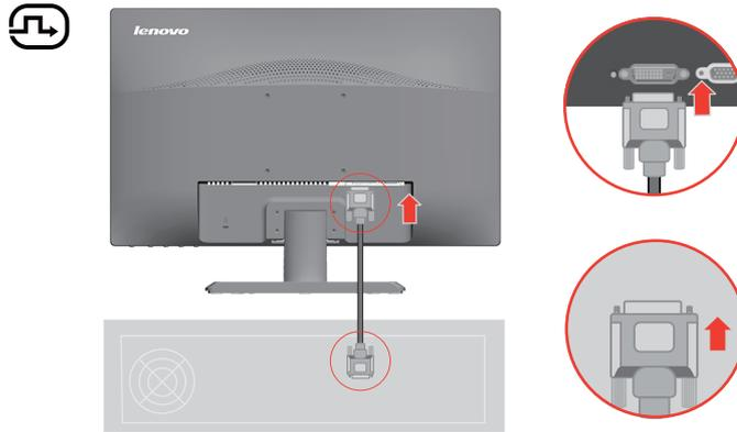
5. Insert the power cord into the monitor, then plug the monitor power cord and the computer cord into grounded electrical outlets.
