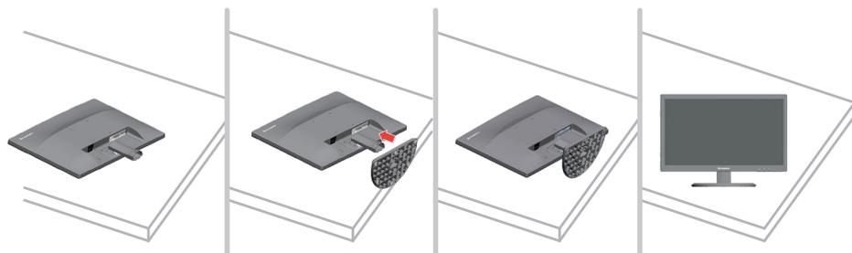
1. Carefully lay the monitor on a flat surface.
