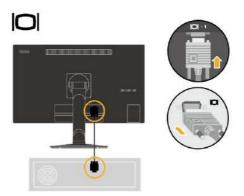
3. Connect one end of the DP cable to the DP connector on the back of the computer, and the other end to the DP connector on the monitor.
