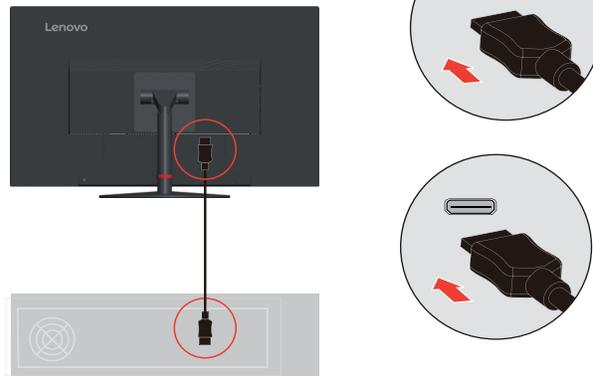
4. Connect one end of the DP cable to the DP connector on the back of the computer, and the other end to the DP connector on the monitor.
