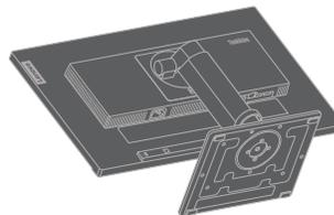
Step 4: Attach the mounting bracket from the VESA compatible wall mounting kit (100mm x100mm distance), VESA Mounting Screw M4 x 10 mm.
