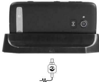
1. Insert the small end
