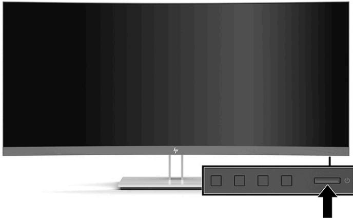
When the monitor is first turned on, a monitor status message displays for five seconds. The message shows which input is the current active signal, the status of the auto-switch source setting (On or Off; default setting is On), the current preset screen resolution, and the recommended preset screen resolution.
