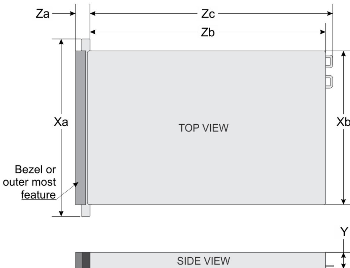
Figure 6. Chassis dimensions
