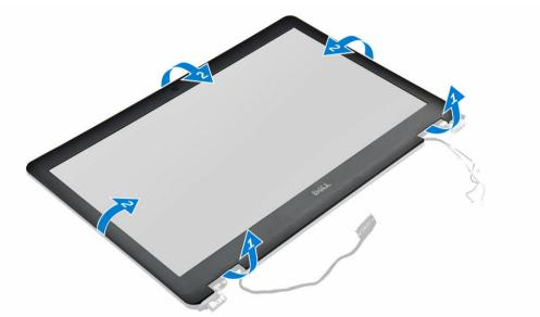
4 Remove the display bezel from the display assembly.
