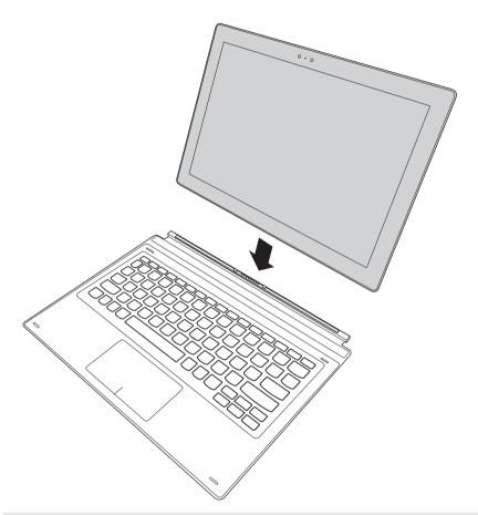
**Note:** Tablet-keyboard folio tongue has strong magnetic force, so as to easily connect with and secure the tablet.
