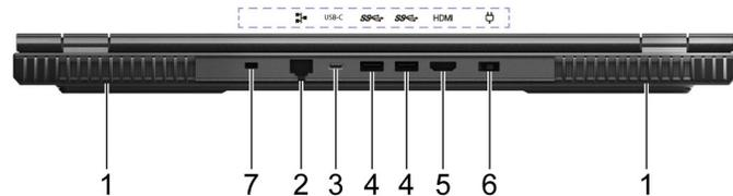
Figure 8. Rear view—17-inch models
