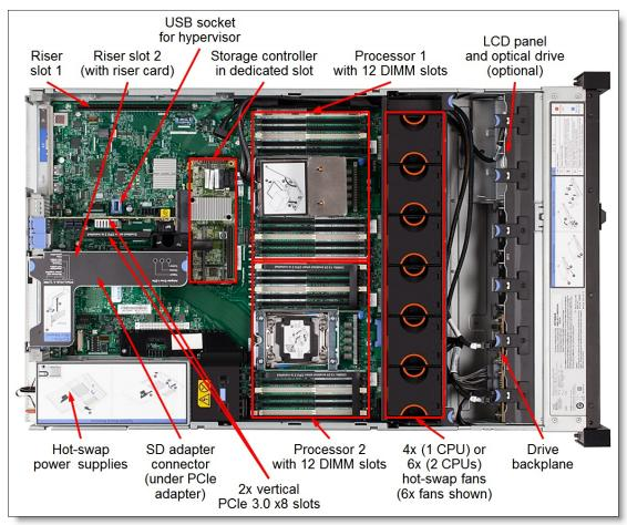
Figure 9. Internal view of the System x3650 M5
