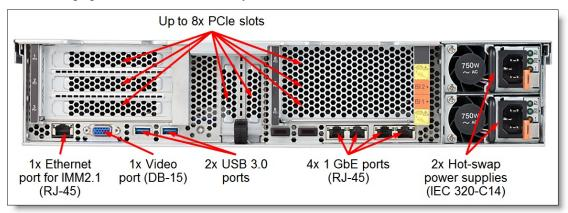
Figure 8. Rear view of the System x3650 M5
