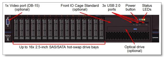
Figure 3. Front view of the System x3650 M5: 16x 2.5-inch drive bays; Front IO Cage Standard (optional)
