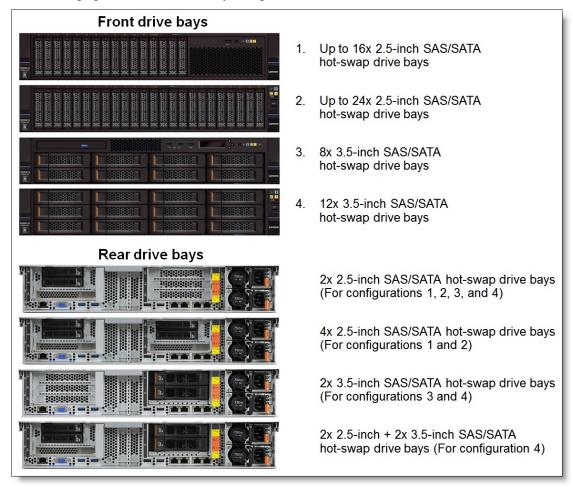
Figure 10. Internal front drive configurations
