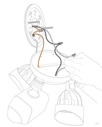
Step 8 - Place Floodlight Cam on the bracket
