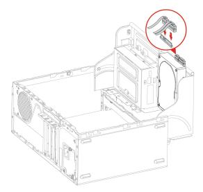
11. Pivot the drive bay assembly downward until it snaps into position.
