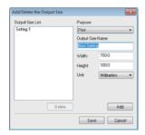
Select [Flexible] to change the output size and the ratio of width to height. Drag the area you want to scan on the preview image or enter values for width and height. If you specify the magnification percentage in the [%] entry field on the right side of the width and height entry fields, the document is enlarged or reduced for scanning.
