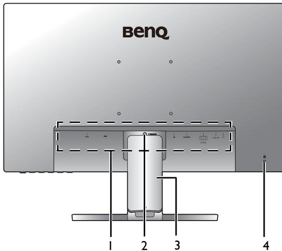
1. Input and output ports (vary by model, see [Input and output ports on page 11](#))
