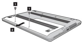
**2** Remove the frame fixing screws **3**.
