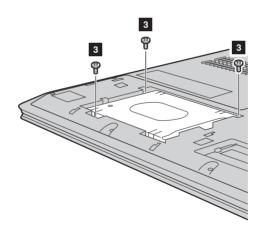
3 Remove the hard disk drive by gently pulling it in the direction of the arrow 4. Take out the hard disk drive secured in a metal frame 5.
