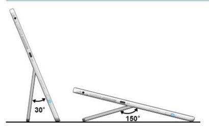
To close the kickstand, push the kickstand against the bottom until it is flush with the bottom.
