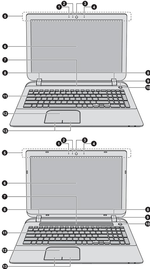
Figure 3-7 Top side of the touch screen model
