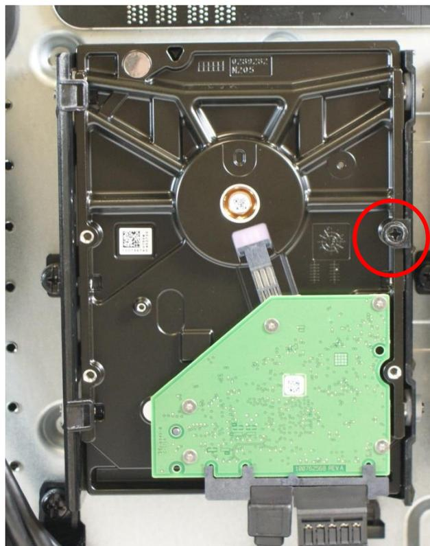
4. Connect the power and data cables to the hard drive.
