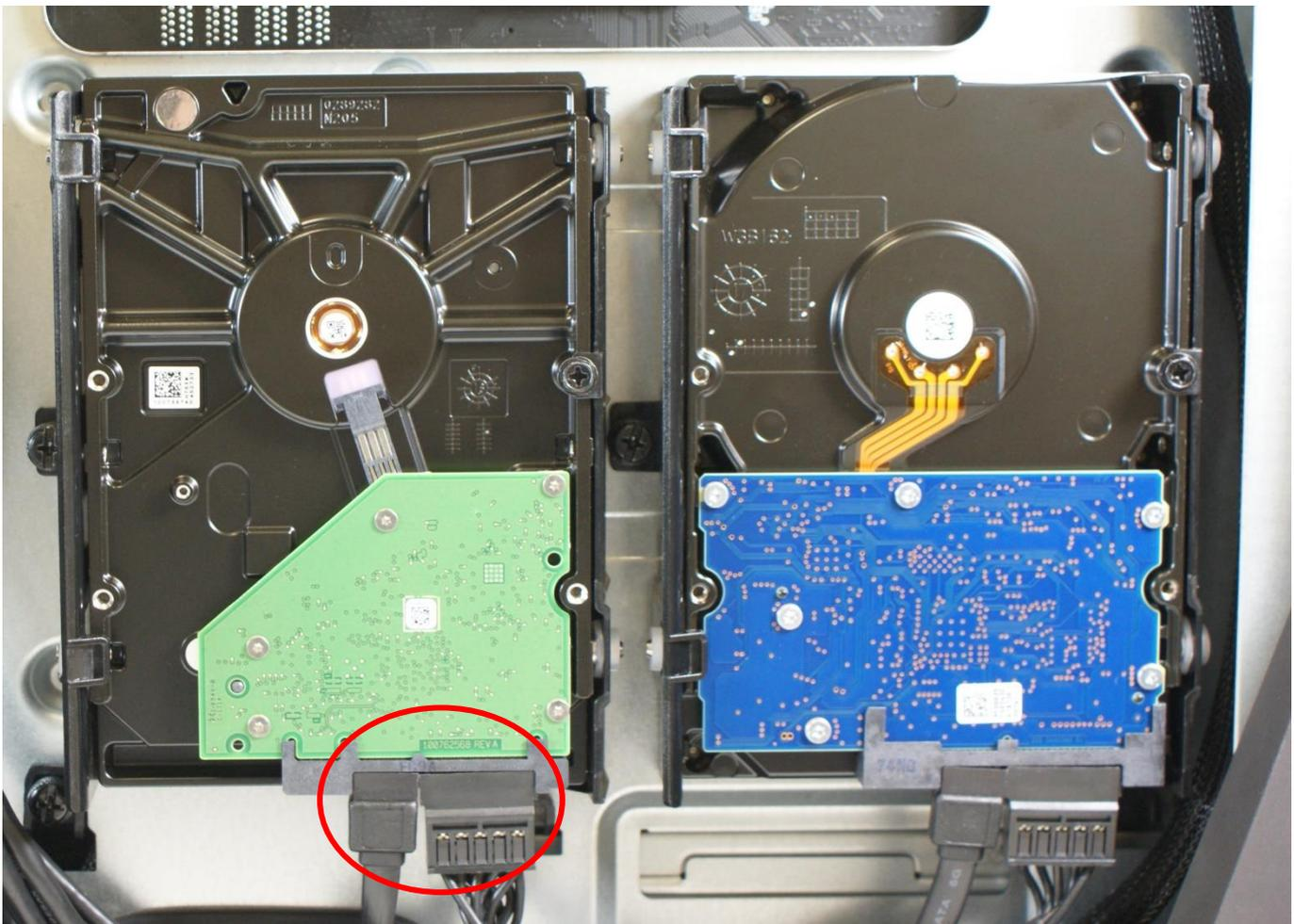
3. Remove the one screws that secure the hard drives to the bracket
