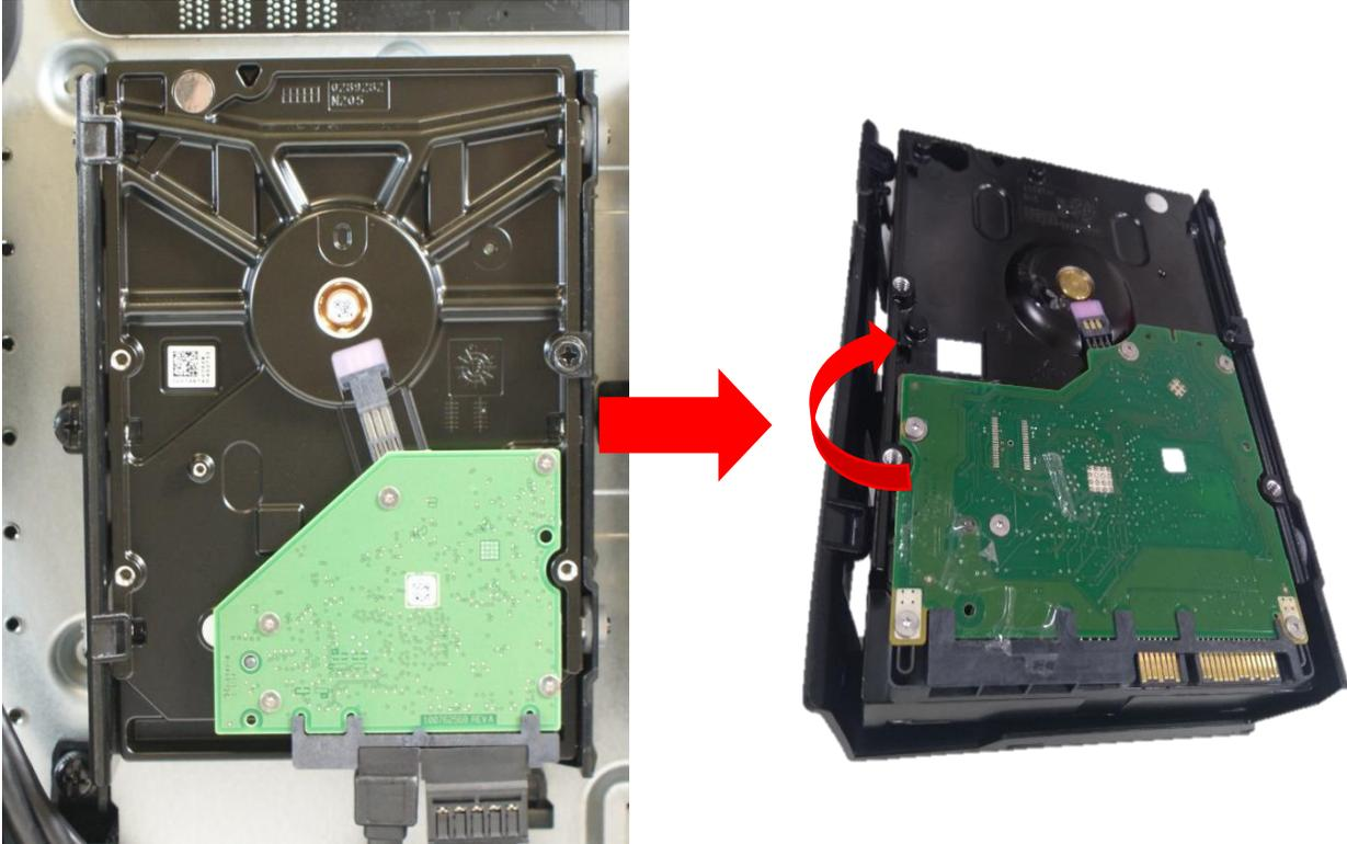
3. Secure the new hard drive with one screw.
