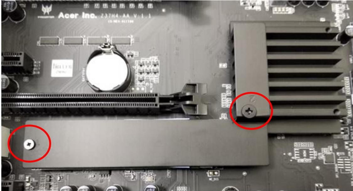
5. Replace the Graphic board. See Installing the Graphic board.
