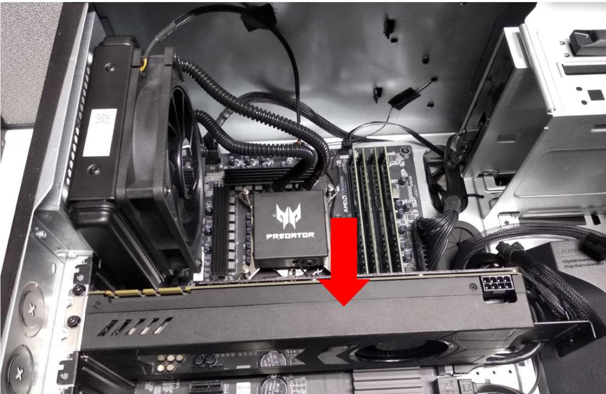
3. Secure the Graphic board with screws.
