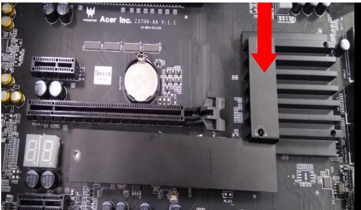
4. Secure the M.2 SSD and thermal module with screws.
