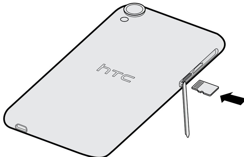
3. To close the slot cover, slightly move it side to side to let the rubber hinge sink down by itself. Then gently press down the cover.
