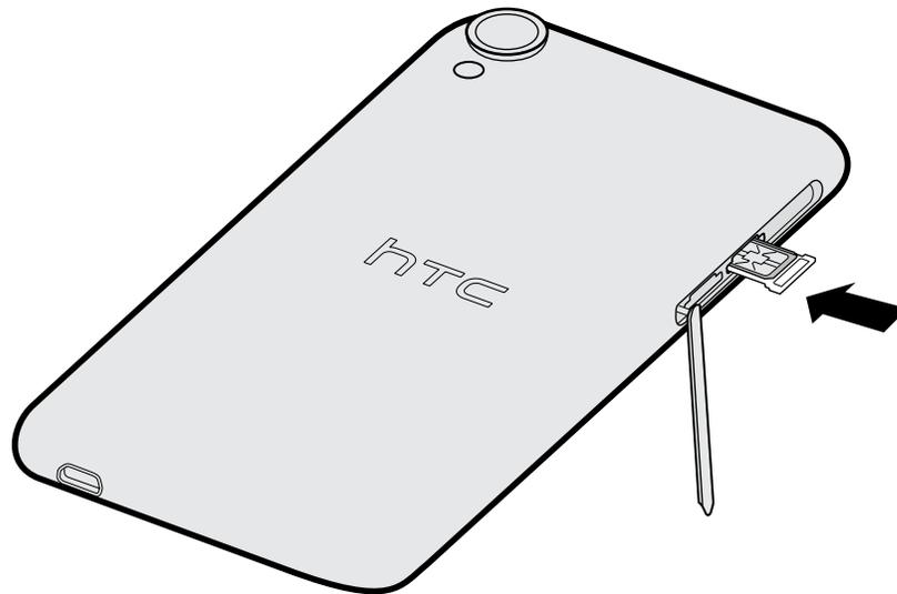
6. To close the slot cover, slide the plastic hinge into the side and press the cover until it clicks into place.
