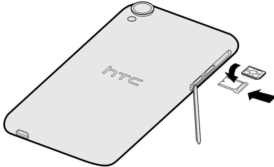
5. Make sure the tray is facing up. Reinsert the tray into the slot.
