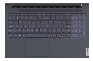
Some Lenovo computers includes a dedicated numeric keypad on the far right of the keyboard. The keypad is used for entering numbers and operators quickly.
