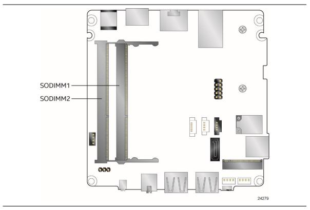
Figure 4. Memory Channel and SO-DIMM Configuration
