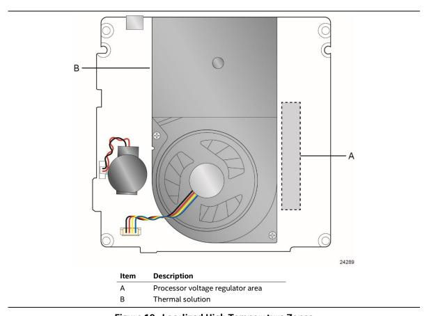
Figure 19. Localized High Temperature Zones
