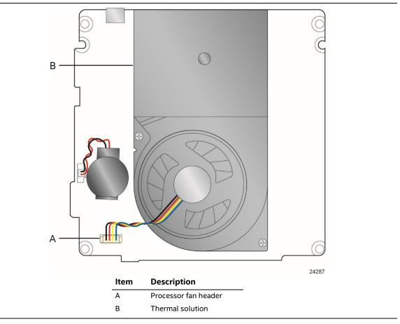
Figure 7. Thermal Solution and Fan Header
