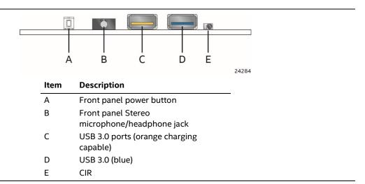
Figure 9. Front Panel Connectors
