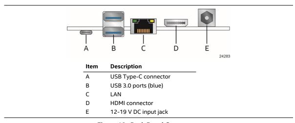
Figure 10. Back Panel Connectors
