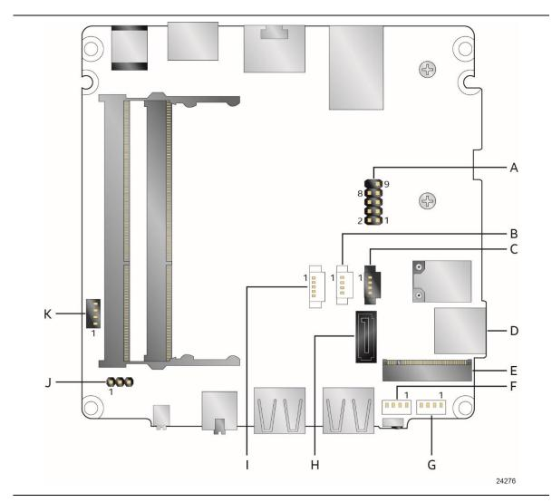
Figure 12. Connectors and Headers (Bottom)
