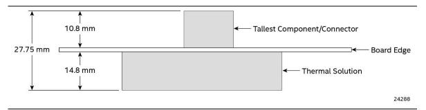
Figure 18. Board Height Dimensions
