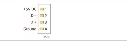
Figure 14. Connection Diagram for the Internal USB 2.0 Single-Port Header (1.25 mm Pitch)
