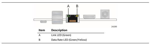
Figure 6. LAN Connector LED Locations
