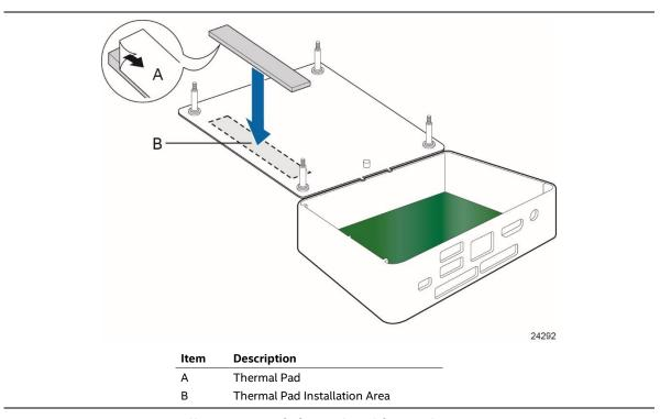
Figure 20. Installation Area of Thermal Pad for Intel NUC Kit NUC7i3BNK
